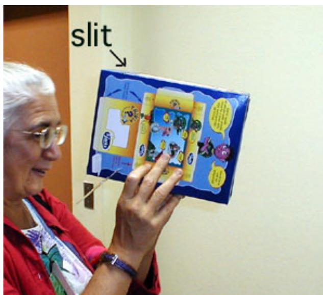
Here is a person looking through the eye hole. they see the slit reflected in the CD. Light from the fluorescent ceiling fixture passes through the slit and is separated into its colors by diffraction off the CD.
