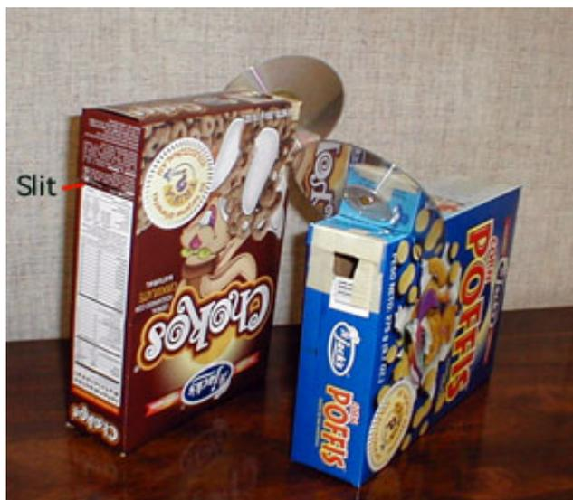
Two views of a cereal box spectrometer. Click on the image to enlarge.
