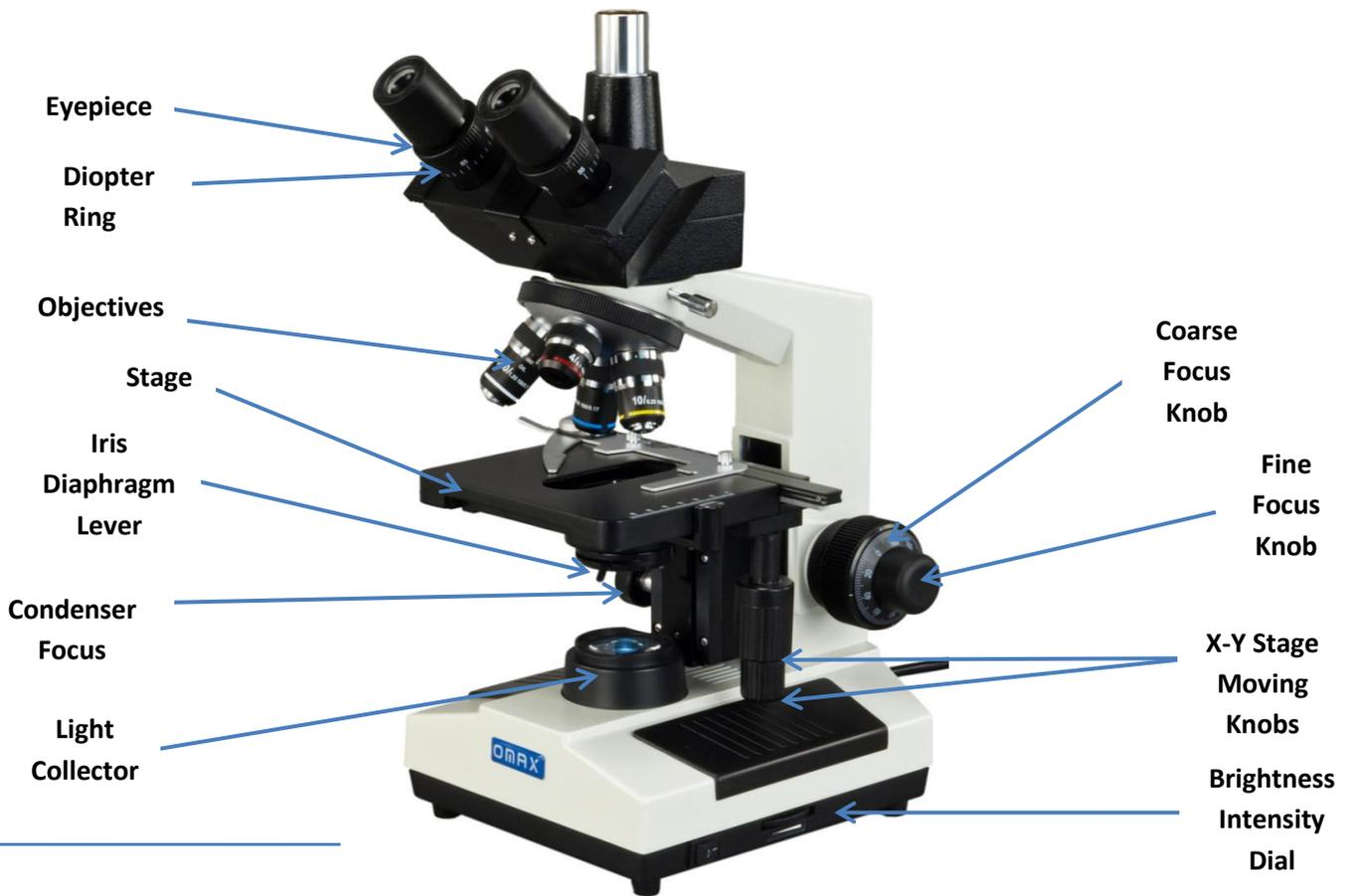
1. **Adjusting the eyepiece:** Using the 10X objective slide the eyepiece tubes in and out and when the left and right fields of view converge completely into one image. Rotate the diopter rings on the eyepiece tubes until its numerical value is the same your interpupillary distance. For example, if there is a distance of 70 then set the diopter at 70.
