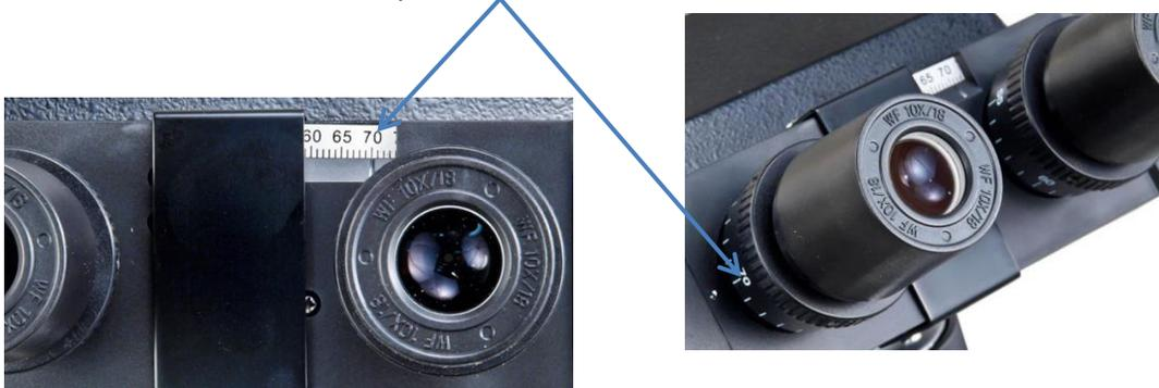
2. **Focusing:** With the 10X objective in position, raise the mechanical stage using the coarse focus knob until the specimen is close to the objective and in focus. Use the fine focus knob to obtain a sharp image. After the image is in focus the 20X objective can be used. **NOTE\*\* To fine focus your picture on the computer screen the fine focus will need to be adjusted approximately 10-11 (on the 10X**
